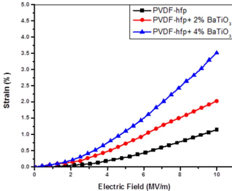
Figure 20. Actuation tensile of electrospun nanofiber mats in a low electric field of up to 10MV/m and in the direction of the electric field or thickness of the sample
