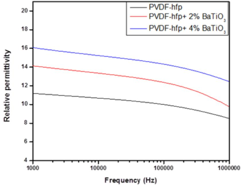
Figure 16. Dielectric spectroscopy of polymer and polymer-ceramic films
