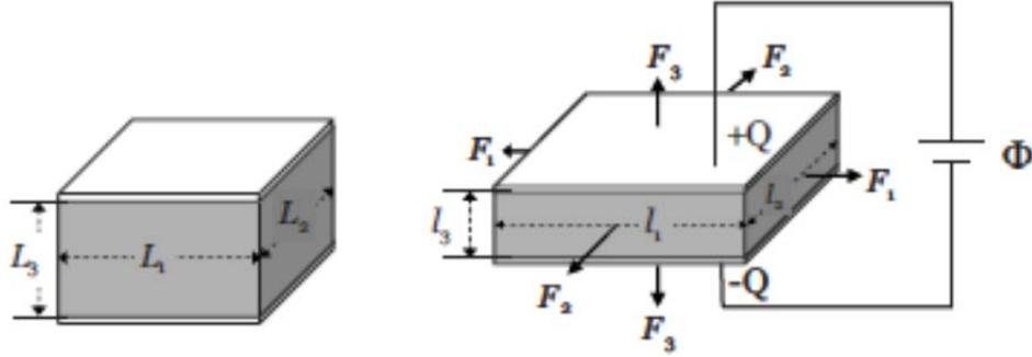
Figure 2. Actuation in the direction of electric field which will result in reduction in thickness of actuator [4]
