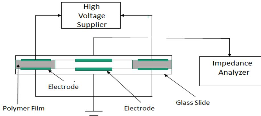
Figure 7. The setup which was used for actuation tensile measurement, with labeled components
