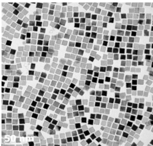
Figure 9. TEM picture of BaTiO<sub>3</sub> nanocubes
