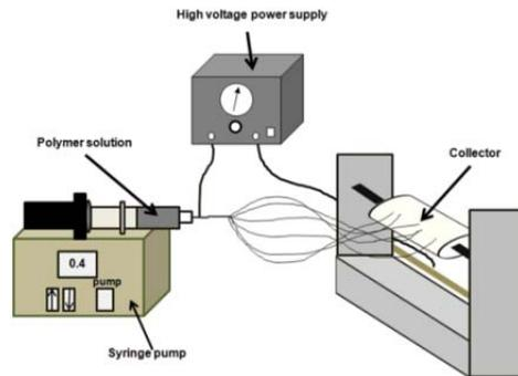
Figure 3. Electrospinning apparatus
