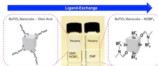
Figure 8. BaTiO<sub>3</sub> cubic colloidal nanocrystals before and after the surface modification with ionic NOBF<sub>4</sub> [52]
