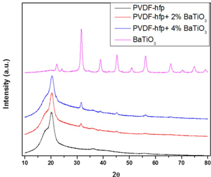
Figure 13. X-ray diffraction (XRD) spectrum of samples showing the crystalline structure of each one
