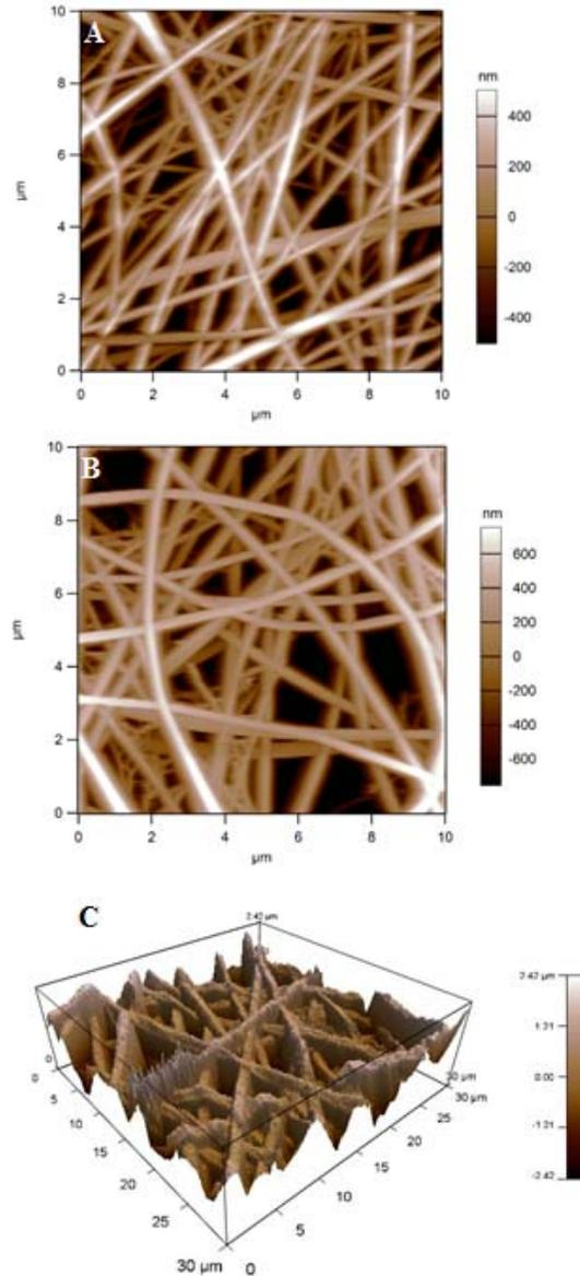
Figure 11. Atomic force microscopy (AFM) images of PVDF-HFP nanofibers showing the morphology of the fibers and the porosity of fiber mats in the absence and the presence of BaTiO<sub>3</sub> colloidal nanocrystals. A) Electrospun PVDF-HFP nanofibers. B) Electrospun PVDF-HFP with 4 wt% BaTiO<sub>3</sub>. C) SEM image showing the topography of fiber mats
