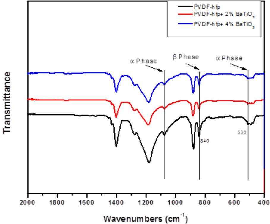
Figure 12. FTIR spectra of samples showing different phases in the nanofibers
