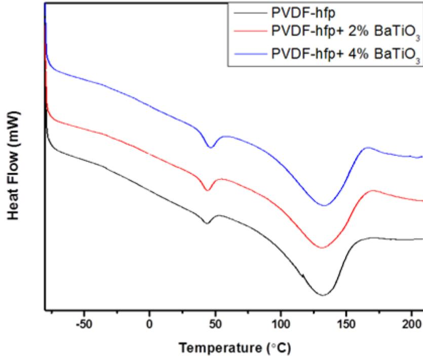
Figure 14. Differential scanning calorimetry (DSC) of polymer-ceramic nanocomposites
