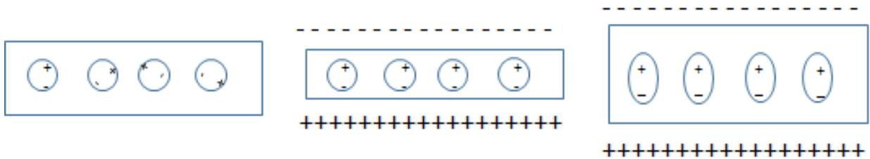
Figure 1. Illustrating the alignment of dipoles inside the sample
