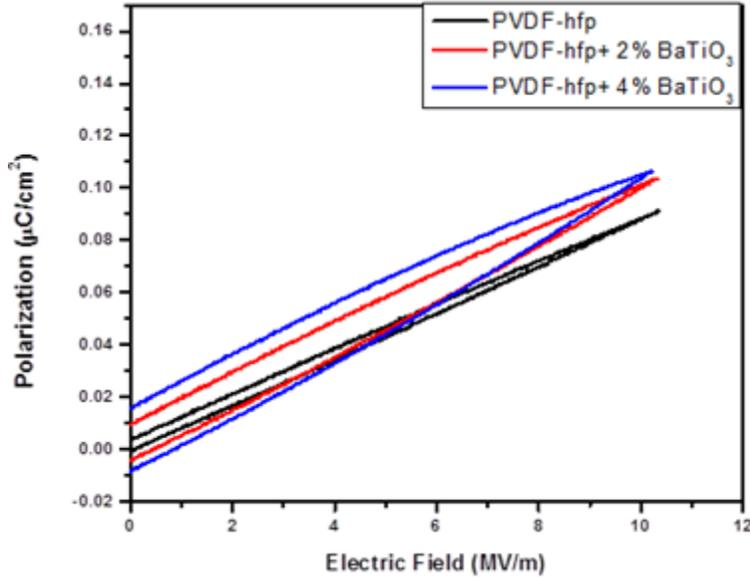
Figure 18. Electric hysteresis loop of the polymer and the nanocomposite samples
