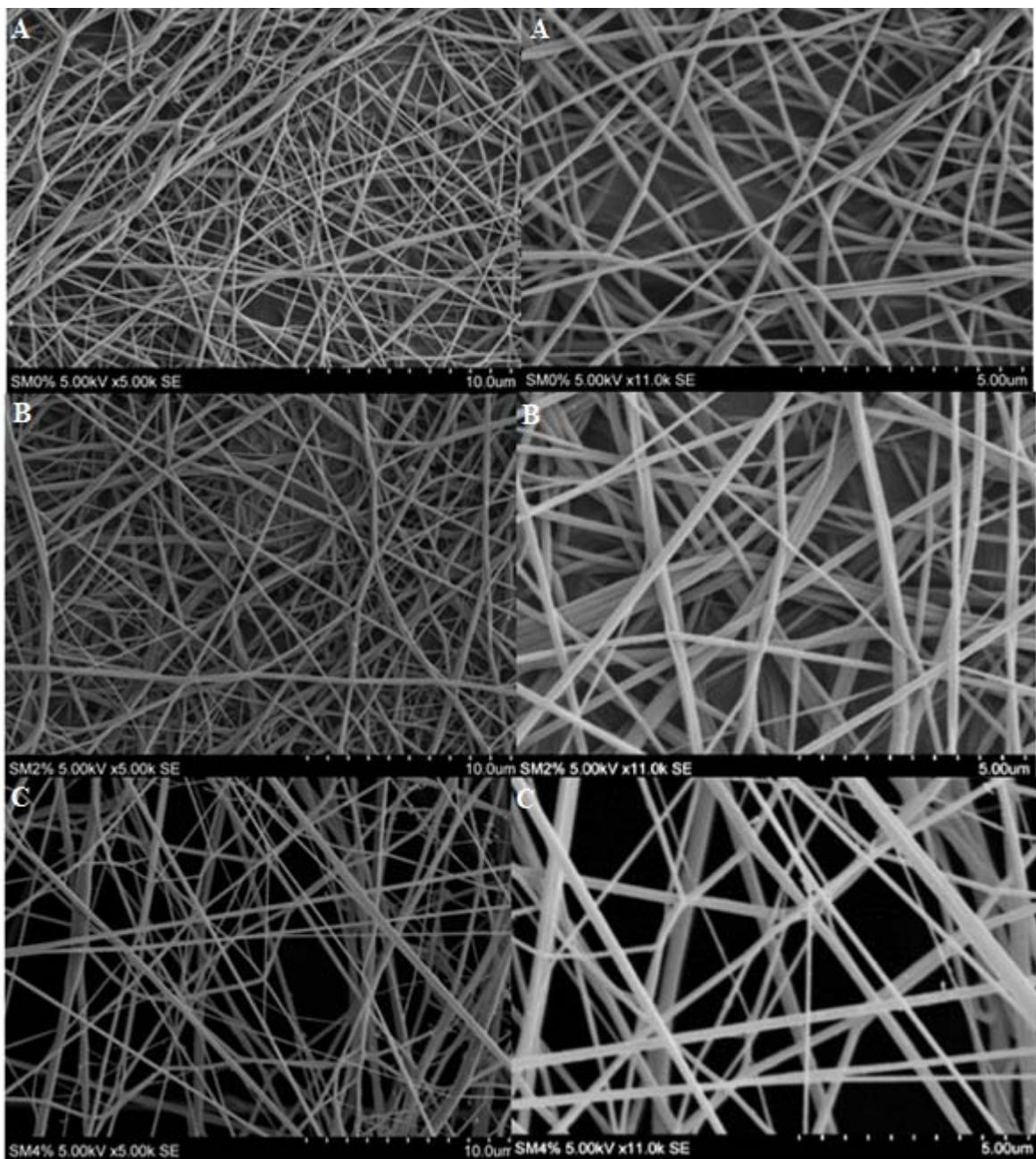
Figure 10. SEM images of PVDF-HFP nanofibers without and with BaTiO<sub>3</sub> colloidal nanocrystals. A) Electrospun PVDF-HFP nanofibers B) Electrospun PVDF-HFP nanocomposite fibers with 2wt% BaTiO<sub>3</sub> C) Electrospun PVDF-HFP nanocomposite fibers containing 4wt% BaTiO<sub>3</sub>
