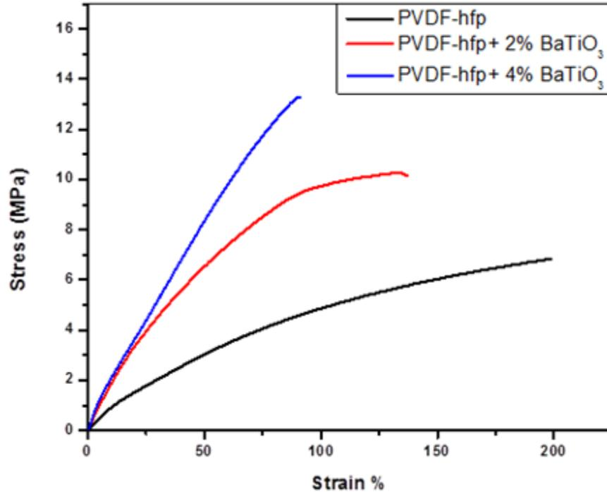
Figure 15. Dynamic mechanical analysis (DMA) of the nanofibers, showing the increase in strength and Young's modulus by increasing the BaTiO<sub>3</sub> content
