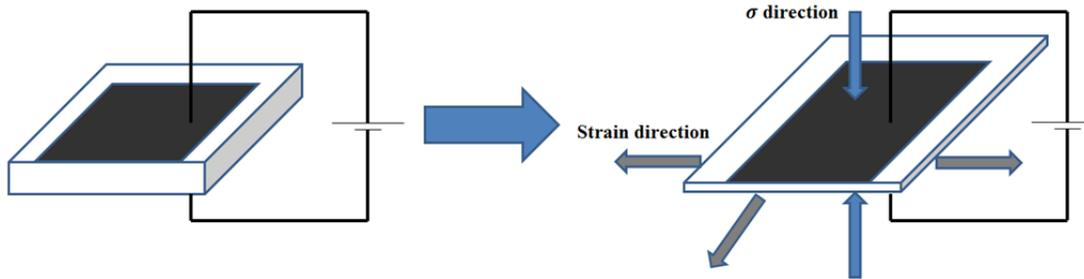
Figure 19. Demonstration of strips used for actuation tensile measurement. Left image shows the sample in absence of electric field and right image is the sample in the electric field undergoing actuation which will result in an increase in area and a decrease in thickness
