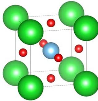
Figure 6. Cubic structure of BaTiO<sub>3</sub> as a perovskite
