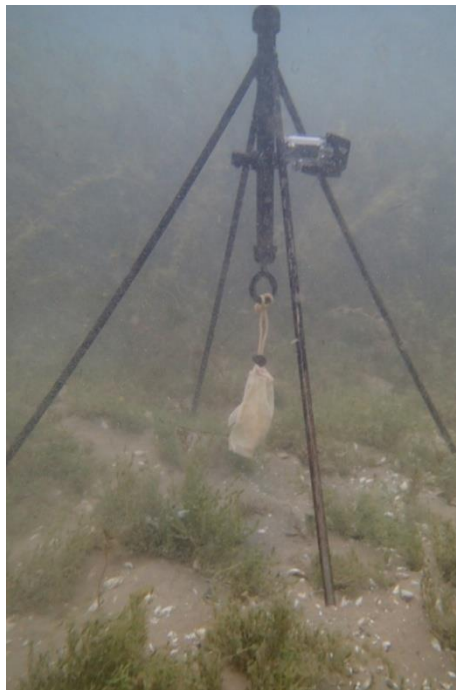
Figure 3.1. The steel rod photoquadrat frame used in Lake Michigan to assess benthic fish abundance. Each quad-pod frame was baited with Lake Trout ( Salvelinus namaycush ) eggs and had a downward facing GoPro ® camera attached to the center.
