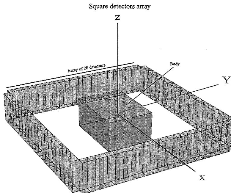
Figure 3.2. The square detector array and the body phantom both are located at the center of the geometry reference frame.
