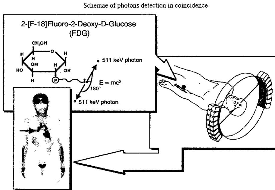
Figure 1.2. Pairs of  $\gamma$ -ray photons are detected in coincidence. Detectors are linked through coincidence circuit to ensure that the pairs are from the same annihilation event. Figure taken from [5, p. 2].
