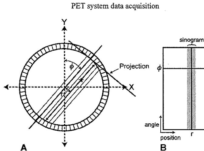
Figure 1.4. Acquisition of data in PET system. Data for all  $r$  and  $\phi$  values that have been acquired in (A) are plotted in polar coordinates  $(r, \phi)$  to produce sinogram indicated by the shaded area (B). Figure taken from [9, p. 14].
