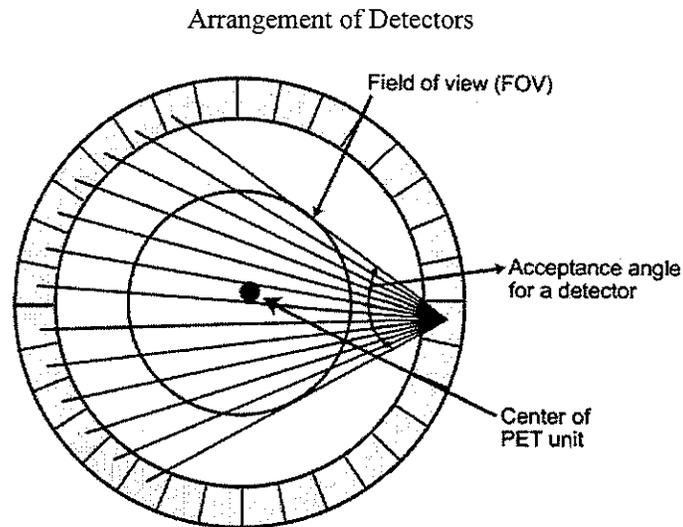
Figure 3.1. Each detector is connected in coincidence with a half total number of detectors in the ring. Figure take from [9, p. 27].
