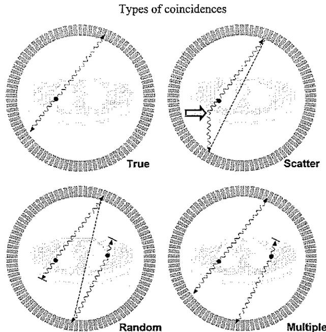
Figure 1.3. Schema of different types of coincidence events registered by PET system using a ring of detectors array. The position of positron annihilation is indicated by the black circle. Figure taken from [10, p. 42]
