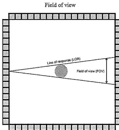
Figure 4.2. Field of view (FOV) for the square array detector. Line of response is the line that connects two detectors in the coincidence circuit.
