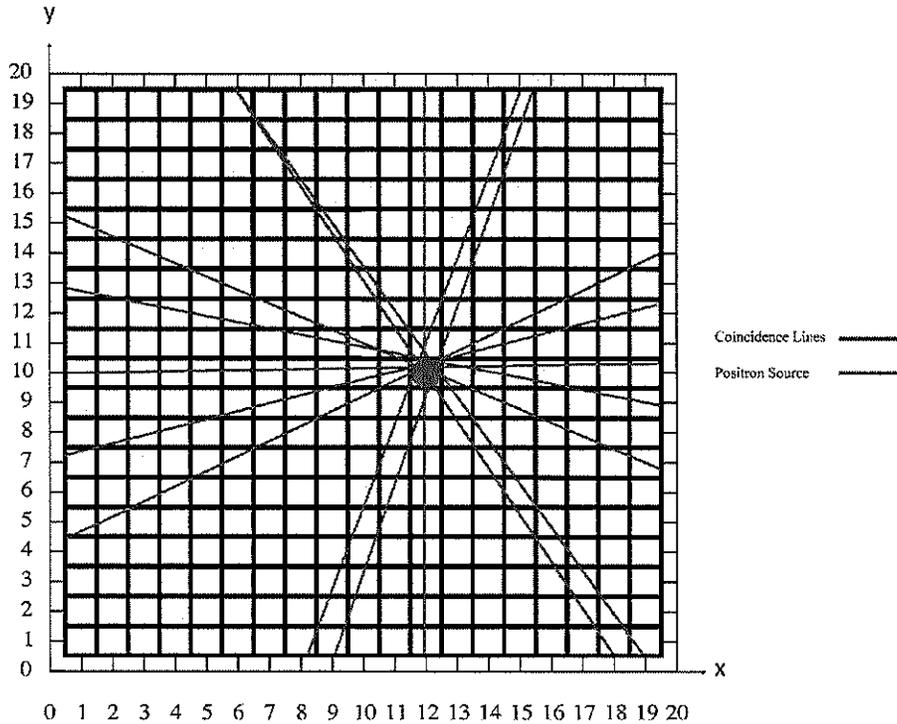
Figure 4.1. Schematic of source position and size reconstruction. Each red line represents the line of response (coincidence event).
