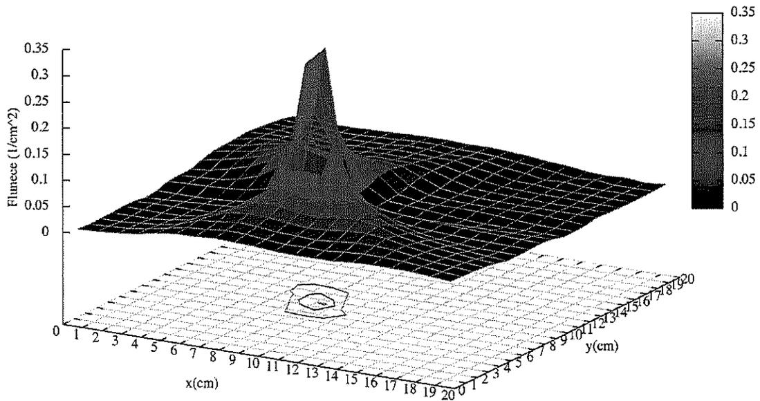
Figure 4.6. Positron sources located at (8.0,8.6,0.0). BGO is used as detector material. The size of the source is estimated by the size of the ring corresponds to the highest peak of the flux distribution. \* 1 division=5 cm
