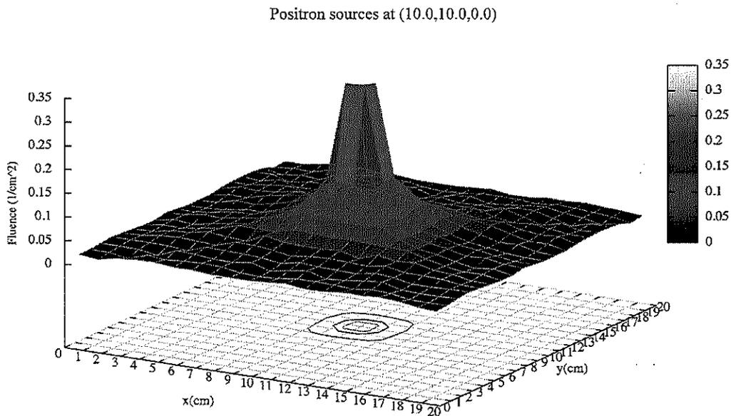
Figure 4.3. Positron sources located at (10.0,10.0,0.0). Silicon is used as detector material. The size of the source is estimated by the size of the ring corresponds to the highest peak of the flux distribution.
