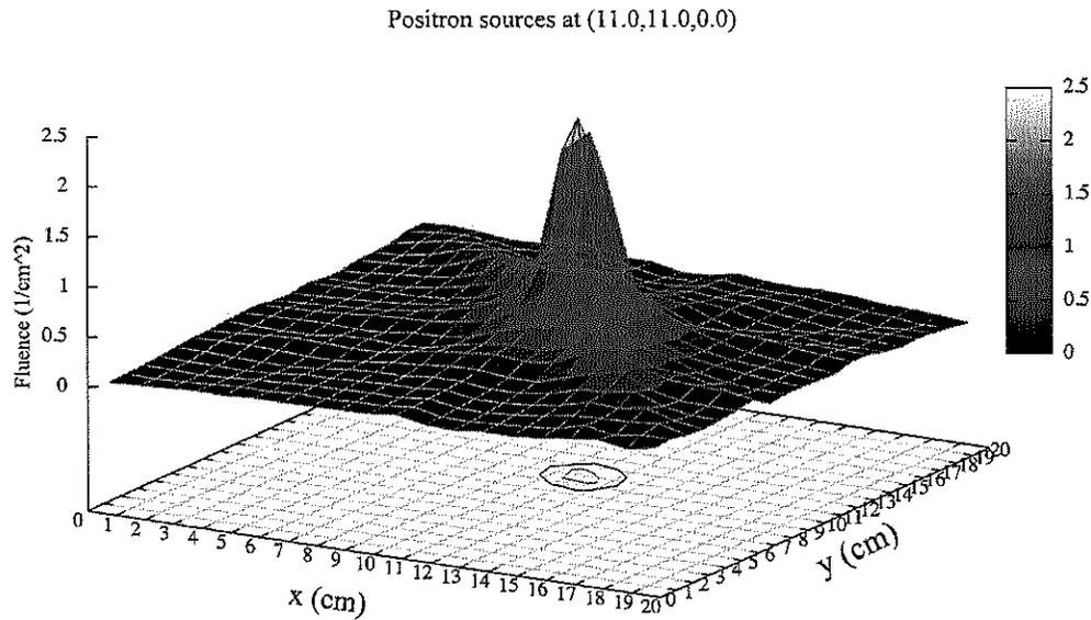
Figure 4.4. Positron sources located at (11.0,11.0,0.0). Silicon is used as detector material. The size of the source is estimated by the size of the ring corresponds to the highest peak of the flux distribution.
