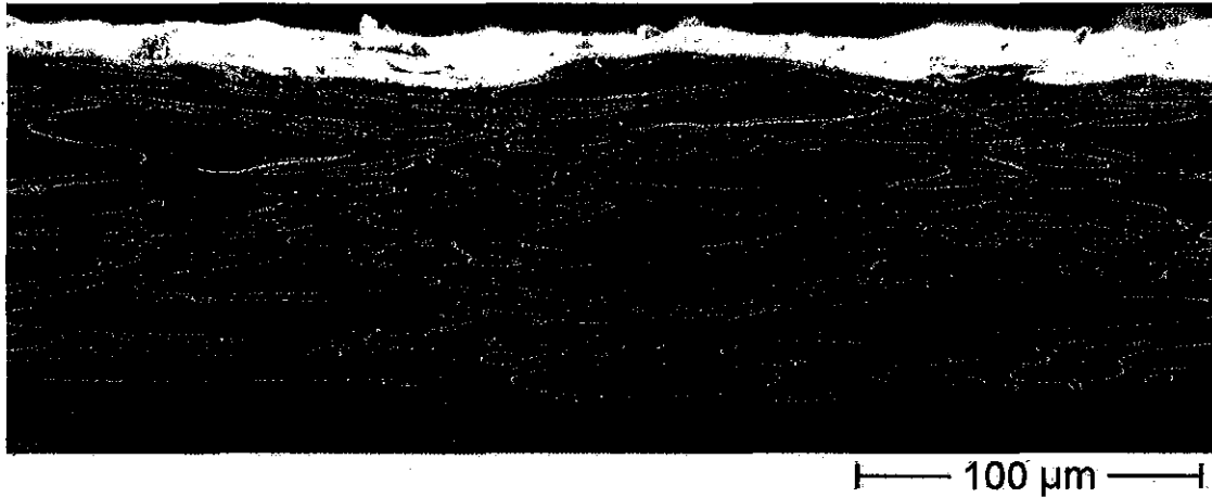
Figure 2.2. Scanning electron micrograph of a cellular polypropylene film from which the thickness parameters s , s_p and the void height distribution n_i were obtained. Best fit ellipses were found using ImageJ.
